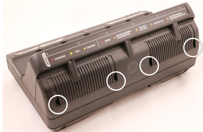
Figure 24: The Four Screws on the Rear Shroud
