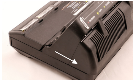
Figure 26: Pocket Insert Screw Removal
