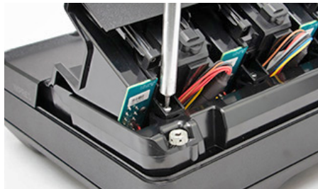
Figure 26: Pocket Insert Screw Removal
